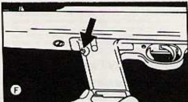
Releasing the clip magazine
